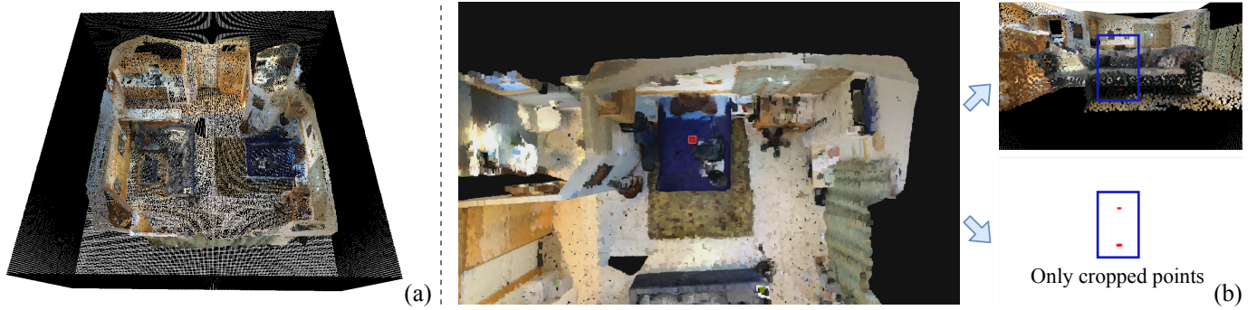
Fig. 2. Demonstration of our labeling process. (a) The labeling tool. We generate dense meshgrids surrounding the scene to help fitting 3D lines. (b) We choose a view to crop the 2D center of object. The cropped points are then used to fit a 3D line. We can repeat this operation and compute the center of object with the two lines.
